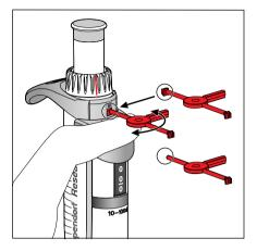
9. Document the changes made and the measurements conducted. Remove the mark on the volume setting ring and the ejector. The red safety plug on the pipette indicates that the Research plus has been adjusted and calibrated by the user.
