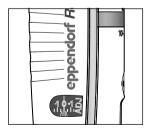
2. Mark the volume setting ring and the ejector with a common mark with a pen. This mark serves as an orientation for factory adjustment changes. When changing the factory adjustment, you can turn the volume setting ring, without the volume display changing. The mark on the volume setting ring and the ejector informs you how far you have moved from the factory setting.
