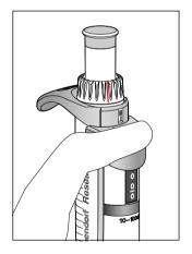
7. If the measured gravimetric values meet your requirements: Slide the locking mechanism up.
