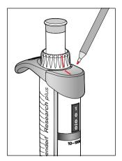
4. Continue to keep the ejector pressed. Insert the safety plug tool such that the counter locking mechanism is pushed down.
