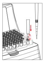
The pipette is only functional if a pipette tip has been attached. You can either attach the pipette tip by hand or directly insert the end of the pipette into a tip held in the tip storage box. If attaching a pipette tip by hand, it must be handled in such a way to avoid contamination and heating of the pipette tip.
