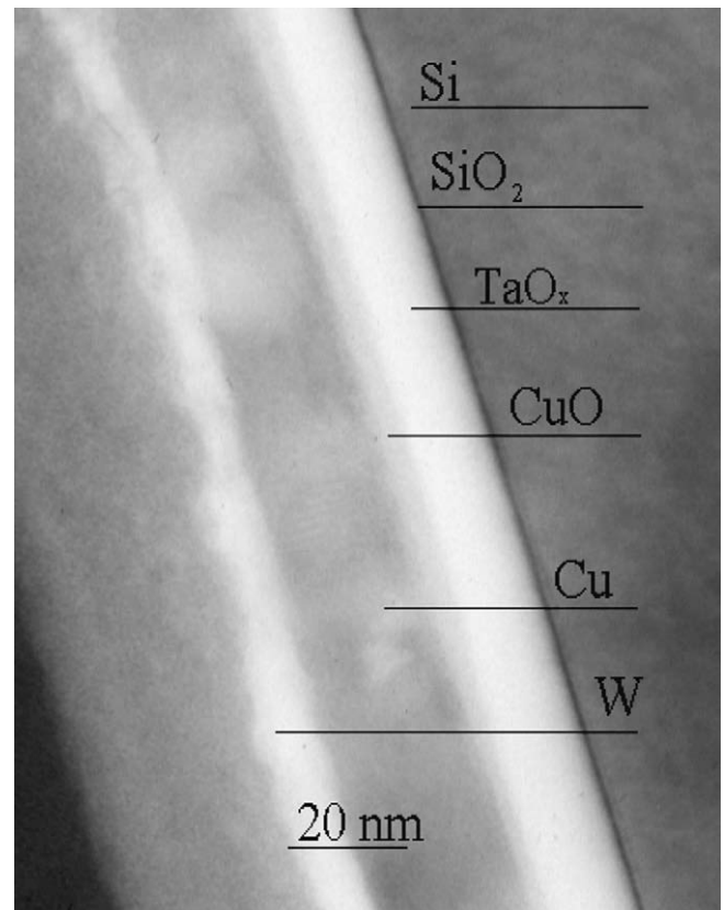
Fig. 2. TEM picture of as-deposited Si/TaO x /Cu/W system.
