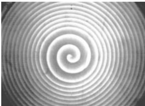
Fig. 2 Evolution of a spiral after the laser beam, focused at the spiral core, has been turned on. The spiral has a diameter of 20.25 mm. Concentrations are: [\text{H}_2\text{SO}_4]_0 = 0.3 \text{ M} , [\text{NaBrO}_3]_0 = 0.40 \text{ M} , [\text{MA}]_0^{\text{A}} = 0.40 \text{ M} , [\text{NaBr}]_0^{\text{A}} = 30 \text{ mM} , [\text{SDS}]_0^{\text{A}} = 0.03 \text{ mM} and [\text{ferroin}]_0^{\text{B}} = 1.0 \text{ mM} . Superscripts A and B designate the reactors into which the chemicals are introduced. MA: malonic acid, SDS: sodium dodecyl sulfate and ferroin: tris(1,10- o -phenanthroline)iron(II) complex ion.
